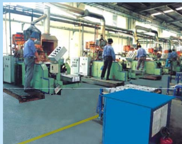
AUTOMATIC GRID CASTING
