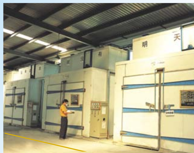
CURING STATIONS ◇Temperature & humidity regulated
